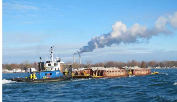
A side-dump barge used to drop rock
