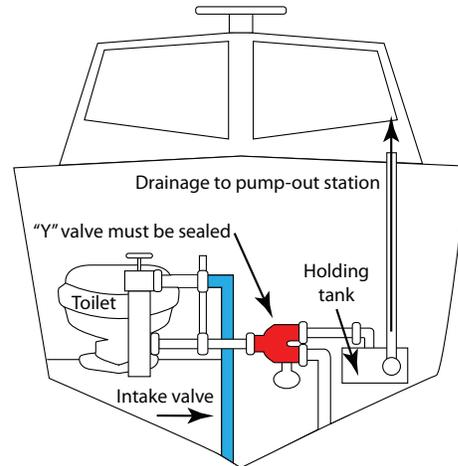
Figure 1: Plumbing connections, such as “Y” valves, can either direct waste into a holding tank, as indicated in the figure above, or overboard. In no discharge zones, the valve must be secured so that it routes waste into a holding tank, rather than into the water.
